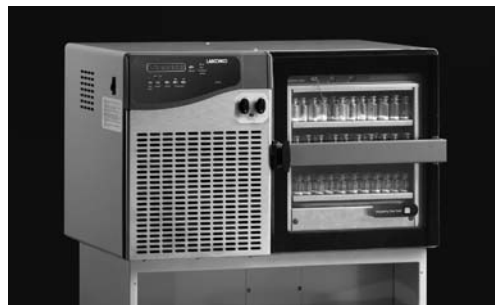
Batch drying in a tray dryer permits precise control of product temperature and heat input.
